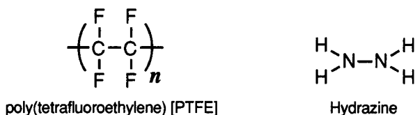
FIGURE 1 Chemical structures of PTFE and hydrazine.
